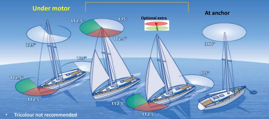
Not compliant for vessels under motor - steaming light must be a --minimum of 1m above sidelights (COLREGS Annex 1 Rule 2 (d)(h))
